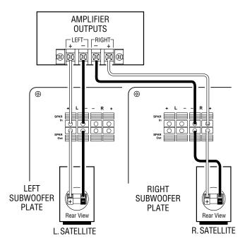
Figure 8. Method when connecting two subwoofers to satellites.
