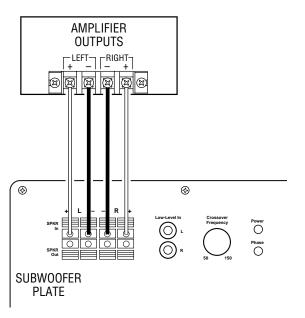
Figure 6. Method when using two subwoofers.
