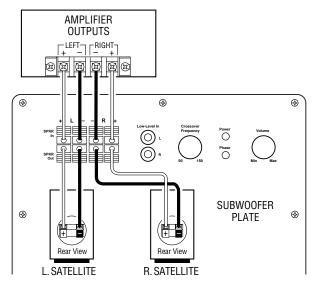
Depending on whether you are using one or two subwoofers, connecting your satellites can be accomplished in one of two ways. If you are using a single subwoofer with a pair of satellites, connect them as shown in Figure 7.
